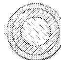
UC m -CONTAINING NANOPARTICLE COVERED WITH METAL NANOSHELL WITH PROTECTIVE COATING LAYER
