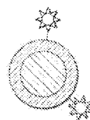
UCm-CONTAINING NANOPARTICLE COVERED WITH METAL NANOSHELL
